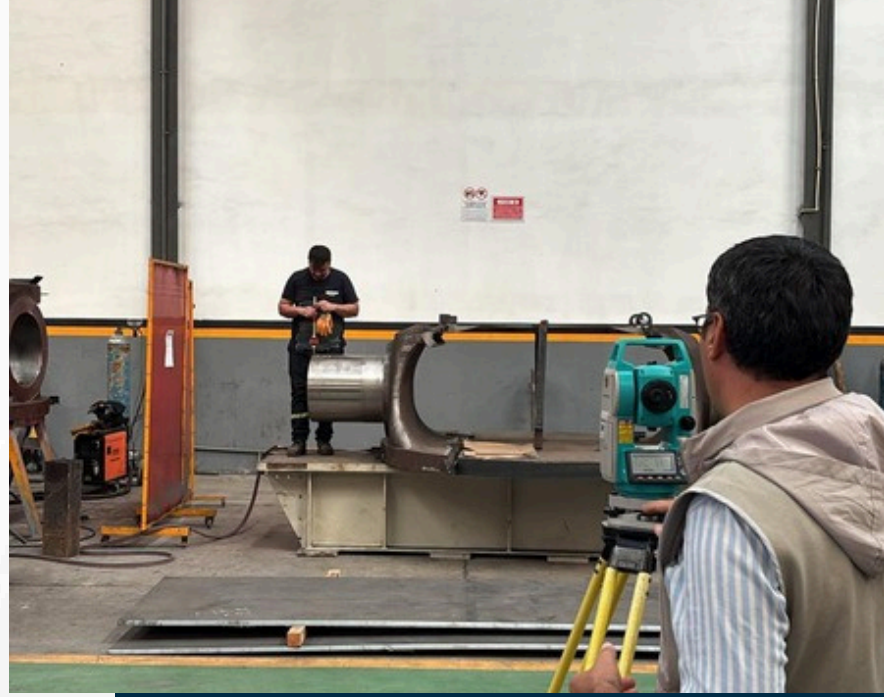
Total Station Controls
